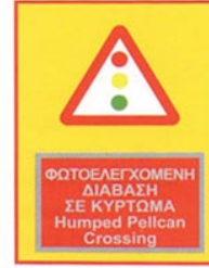
Warning of pelican crossing with road humps
