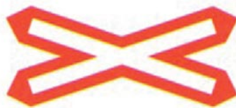
Level crossing without barrier
