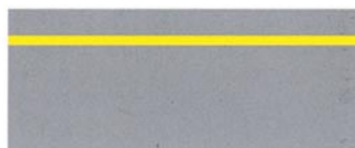
Single yellow line: depicts the side of the carriageway, no parking
